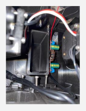
Pictured is the attachment for the raspberry pi that fits into the 70mm x 70mm modular base. The center modular base is also 70mm x 70mm for consistency.
