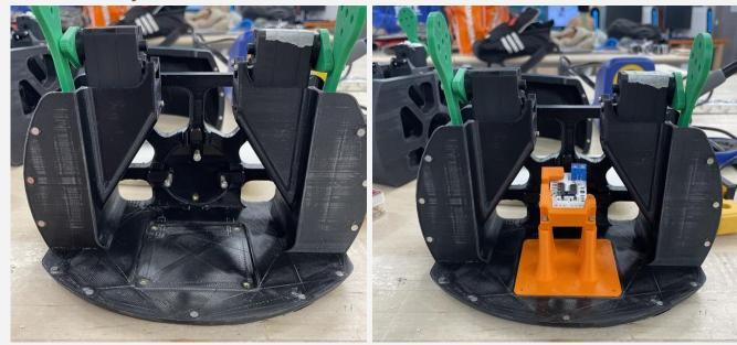
The front, center, and rear body parts have a mounting plate which allows the orange section to be screwed into place. The raspberry pi, servo controller, battery, and DC converter are all attached through this system. The beauty is that if I ever need to change battery systems, or controller boards, I can simply unscrew the part from the mounting plate and add the new design.
